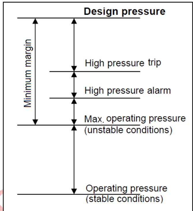
Figure 1 – Margins between operating and design pressure
