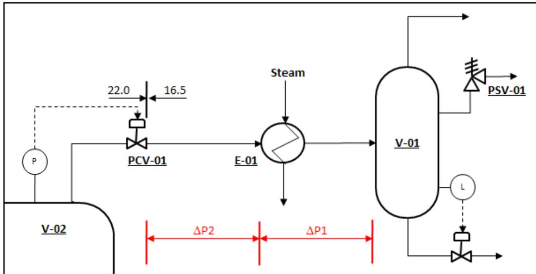
**Figure 3** – A typical system where LP side of heat exchanger is designed for tube rupture
