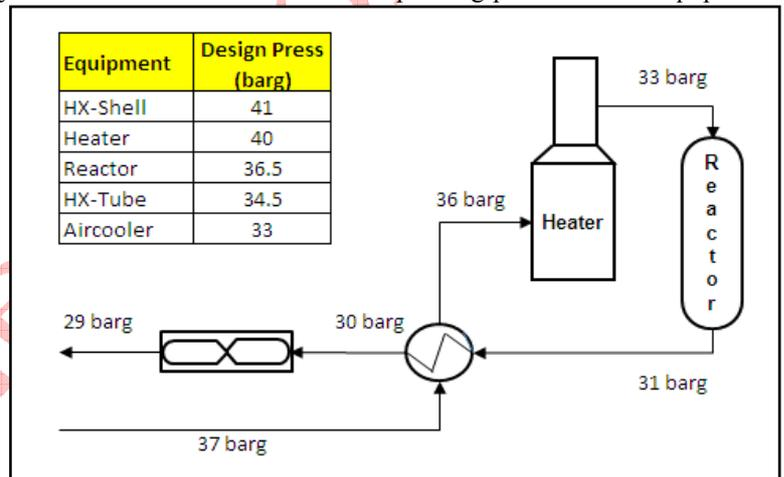
**Figure 2** – Design pressure profile for heat exchangers on a gas route
