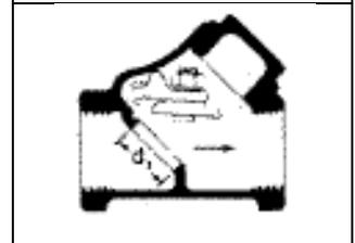
**Figure 6 – Inclined seat swing check valve**
