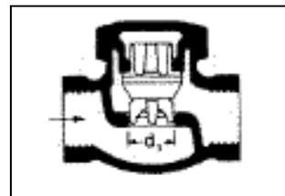
**Figure 8** - Piston check valve – horizontal seat
