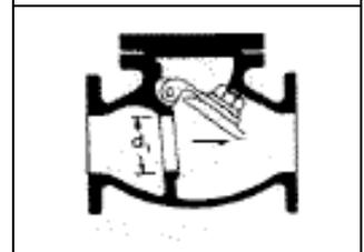
**Figure 7 - Vertical seat swing check valve**
