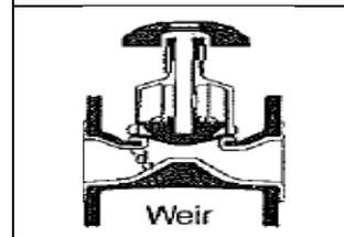
**Figure 12** - Weir type diaphragm valve
