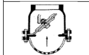
**Figure 11** - Hinged disc foot valve
