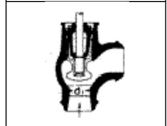
**Figure 5 - Tapered seat angle valve**
