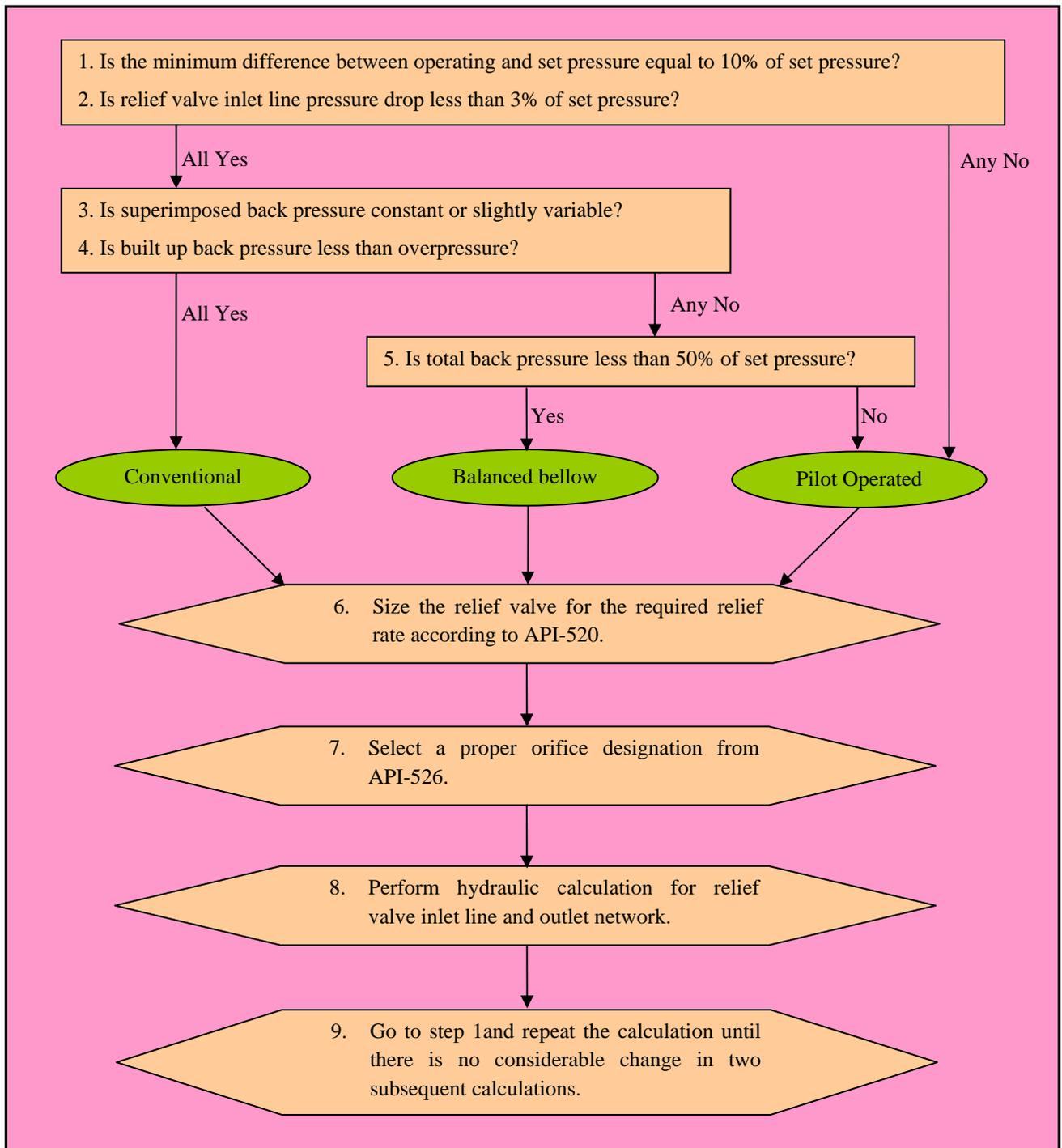
**Figure 1** – Relief Valve Selection Flowchart
