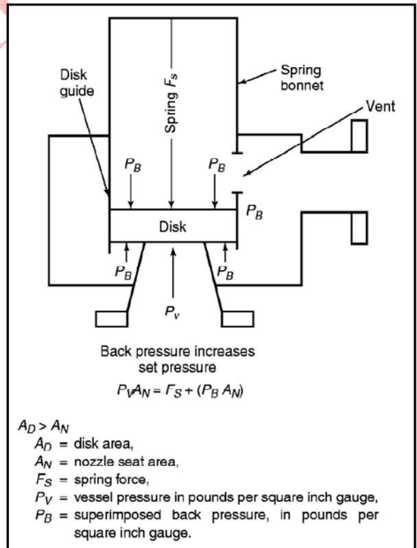
**Figure 2** – The Effect of Superimposed Backpressure on the Opening Pressure of Conventional Relief Valve
