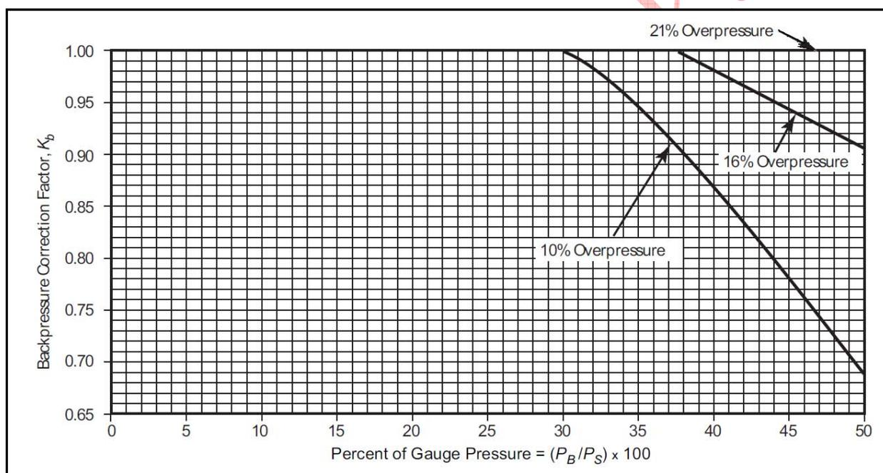
**Figure 3** - The Effect of Backpressure on the Capacity of Balanced Bellows Relief Valve (Gas Service)
