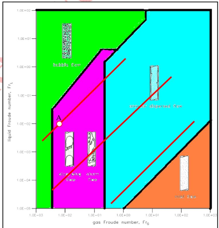
Figure 2 –Two phase flow map for vertical (upward) pipe
