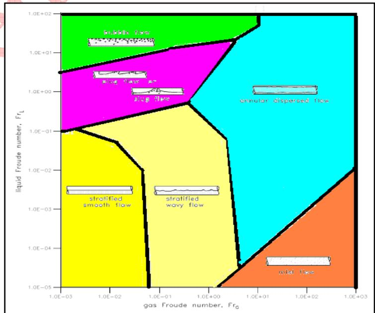
Figure 1 – Two phase flow map for horizontal pipe
