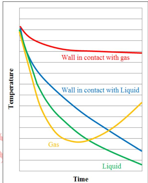
Figure 1 – Typical trend of system temperatures
